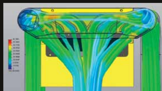
Air purge designed with Computational Fluid Dynamics
